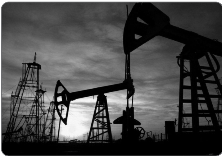
Machines called pumpjacks are used to pump oil out of the ground.
